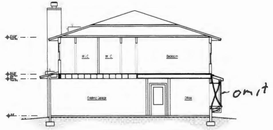
Building Section SCALE 1/4" = 1'-0"
