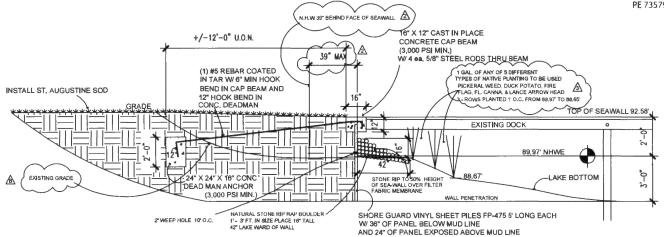
ENGINEER NOTE A CONCAVED WALL WILL FUNNEL ALL THE WAVES ENERGY TO THE ENTER WHICH WILL CAUSE WAVES TO CRASH INTO EACH OTHER, AND CAUSE WATER TO SPLASH ABOVE WALL, IT WILL ALSO CAUSE EXCESSIVE LAKE WEED DEBRIS COLLECT IN CENTER
