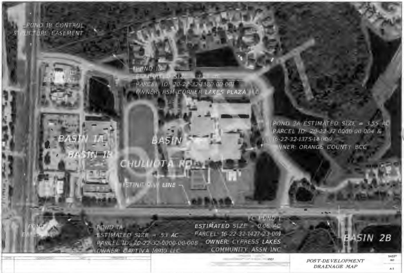
Figure 7-2 – Post Development Drainage Map
