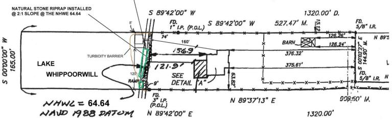
THIS IS TO CERTIFY THE LOCATION OF THE NHWL WAS LOCATED ON 10-6-2014 USING ORANGE COUNTY BENCH MARK C-1134031 NAVD 1988 DATUM TO DETERMINE THE NHWL IN RECATION TO THE EXISTING BUILDING AND PROPOSED REFIDENCE'S POOL
