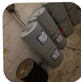
> 25 gallons stored outside of cabinet
