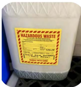
Hazardous Waste labeled but hazard not identified
