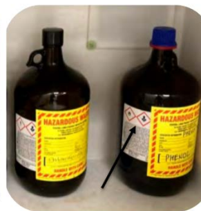
Hazardous Waste label with hazards identified
