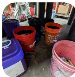
Unlabeled and full used oil containers stored under table
