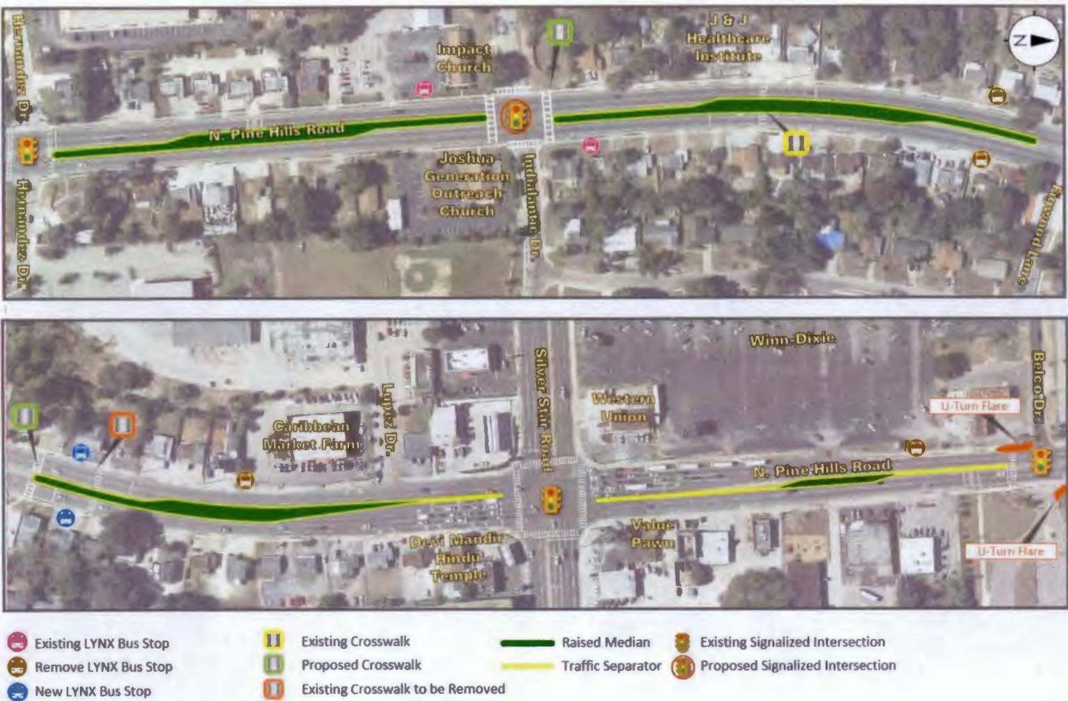
Figure 7.5 (continued): Build Alternative, Raised Median
