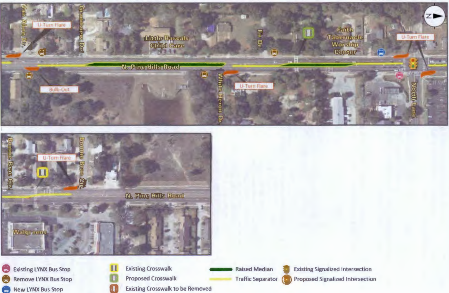
Figure 7.5 (continued): Build Alternative, Raised Median
