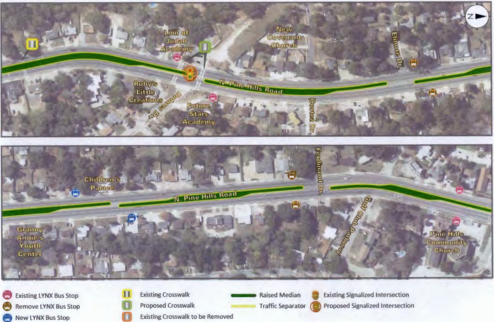
Figure 7.5 (continued): Build Alternative, Raised Median
