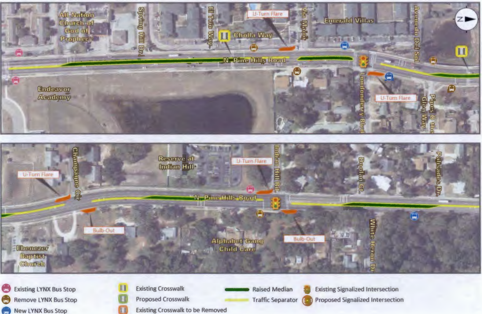
Figure 7.5 (continued): Build Alternative, Raised Median
