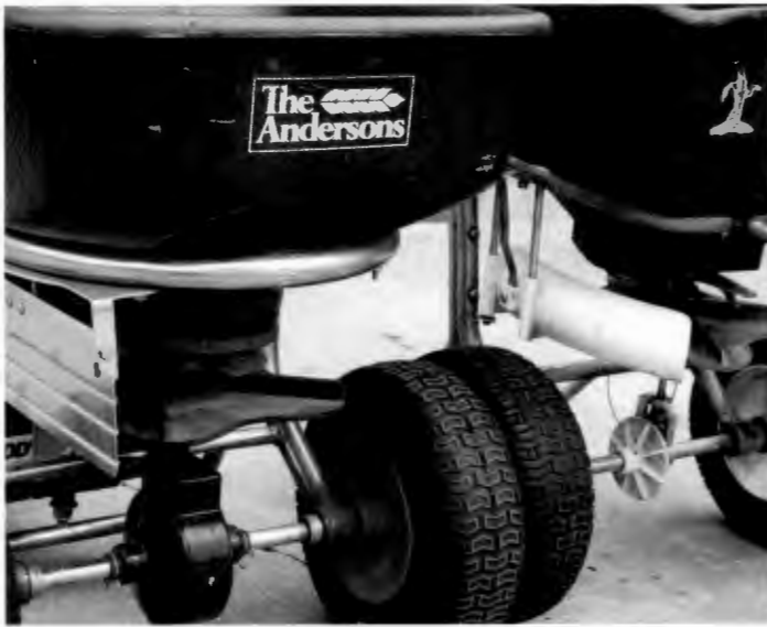
Figure 21. Spreaders with deflector shields.
