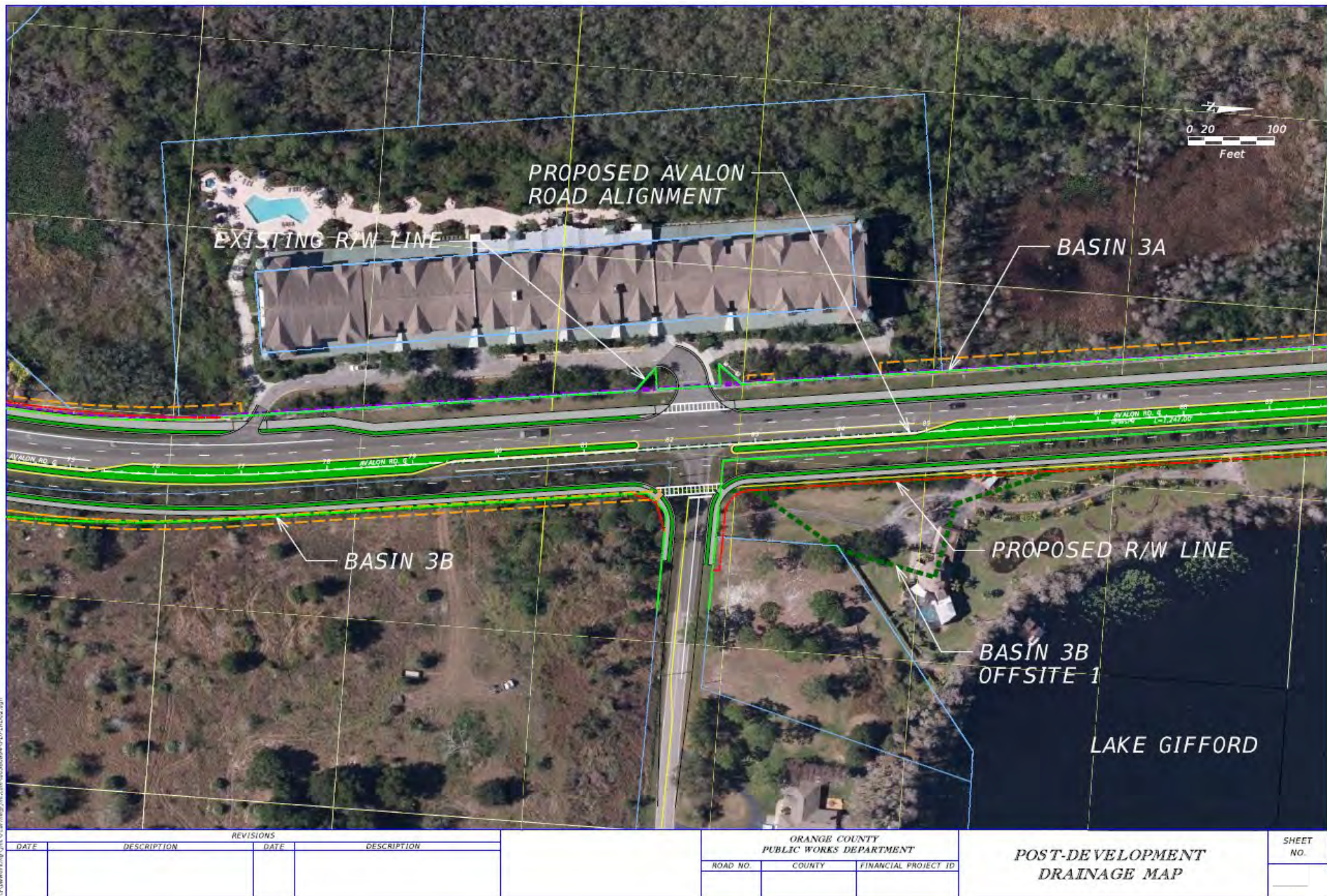
Figure 7-2 – Post Development Drainage Map
