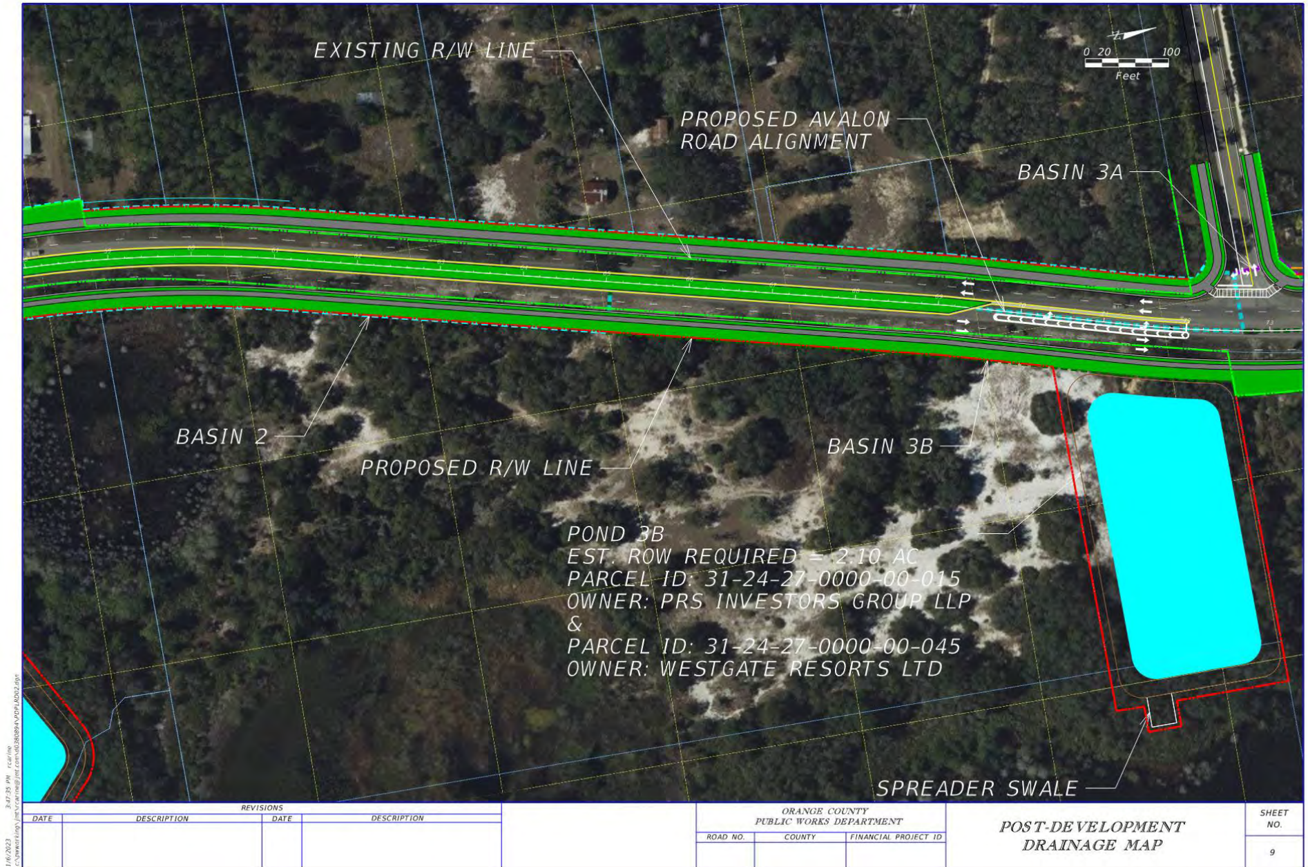
Figure 7-2 – Post Development Drainage Map
