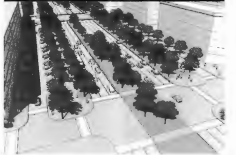
Figure (14). Multiway Boulevard using Frontage Road
