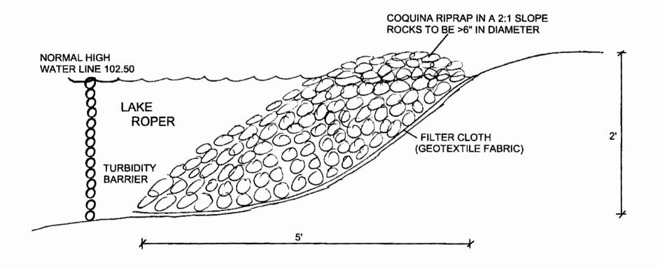
ANY AQUATIC VEGETATION THAT EXISTS IN THE LOCATION OF THE PROPOSED RIPRAP REVETMENT WILL BE CAREFULLY RELOCATED WATERWARD OF THE RIPRAP AND ANCHORED UNTIL THE ROOTS ARE RE-ESTABLISHED.
