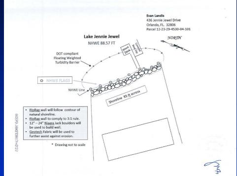
Evan Landis 436 Jennie Jewel Drive **Cross Section** Orlando, FL. 32806 **RipRap Seawall** NHWE 88.57 Geotech Ground level NHWE FLAGS Fabric shown in picture River Jack stones ranging in size from 8"-24". Stones will be placed along natural contour of existing shoreline, with the HEIGHTS being no taller than 1 foot. Shoreline already has 10' drop off from property due to erosion. 3' FT 0CEP0 JAN272017PH2:22 Waterline \* Drawing not to scale Geotech fabric will be anchored at both ends.
