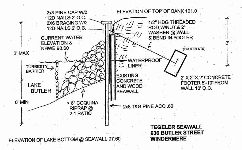
SEAWALL MATERIAL WILL BE EMBEDDED TO JUST BELOW THE LAKE BOTTOM AROUND THE CYPRESS TREES TO MINIMIZE THE IMPACT TO THE TREES. WATERPROOF BARRIER AND RIP RAP WILL INSURE THAT EROSION UNDER THE WALL DOES NOT OCCUR.
