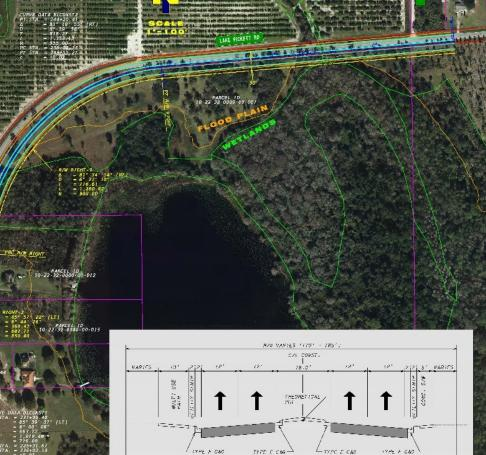
TYPICAL SECTION NO. 2 DESIGN SPEED 40 MPH
