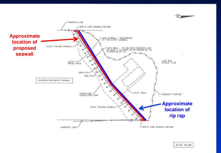
NOTES: CDM - CONCRETE DEADMAM 2X2X2 TBR - TIEBACK ROD @ 10 D.C. MAX. #5 REBAR
