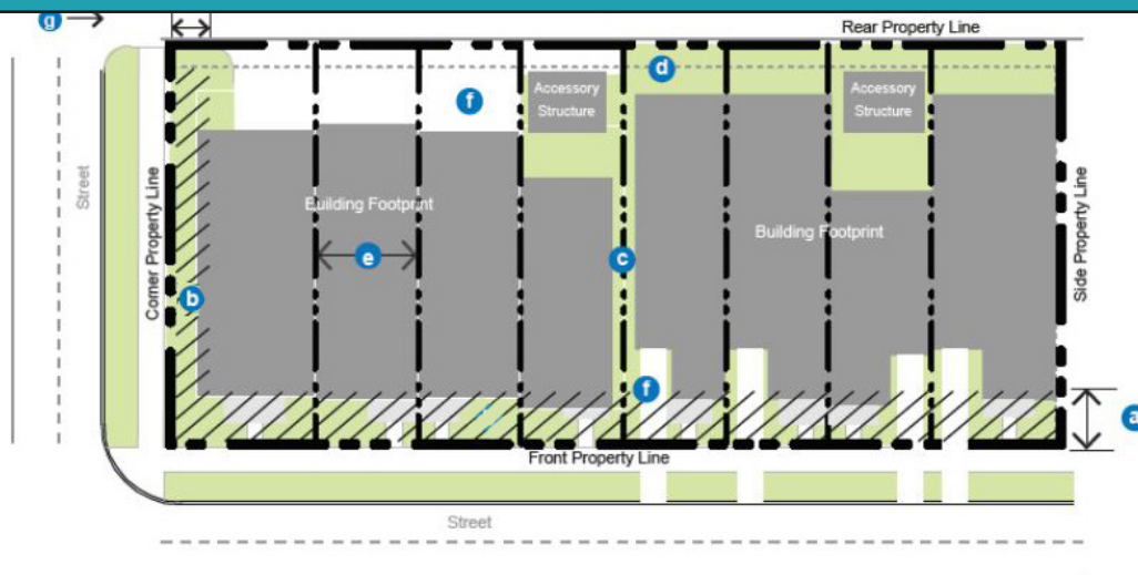
Figure (SB3). Residential Building Siting with Rear Access Attached Garage
